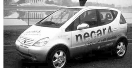
Fig. 9. DaimlerChrysler NECAR 4, powered by a PEMFC and fuelled by pure hydrogen.
